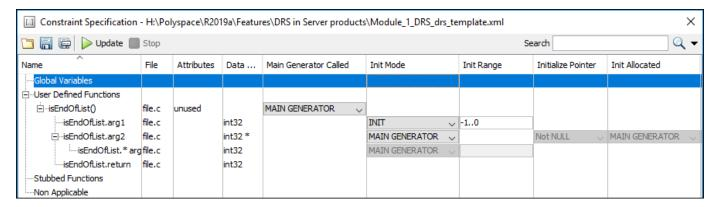
This table describes the various columns in the **Constraint Specification** window. If you directly edit the constraint XML file to specify a constraint (for instance, in the Polyspace Server products), this table also shows the correspondence between columns in the user interface and entries in the XML file. The XML entry highlighted in bold appears in the corresponding column of the **Constraint Specification** window.
