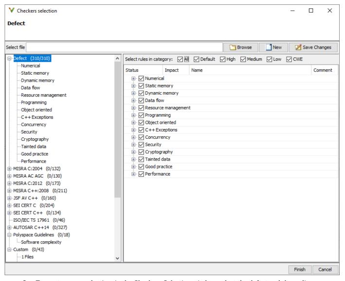
2 To create a new selection, in the Checkers Selection window, select the defect and the coding rule checkers that you want to activate. To modify an existing selection, click **Browse**, navigate to the existing checkers file and then make your selection.
