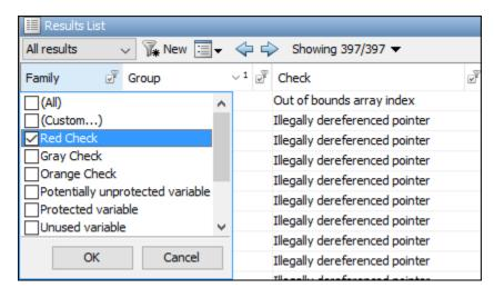
You can filter using the columns on the **Results List** pane. Click the icon on the column headers to see the available filters. For instance:
