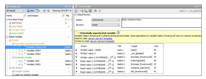
The Code Prover analysis exhaustively checks if shared global variables are protected from concurrent access. The analysis reports variables that are definitely protected in green and variables that might be unprotected in orange. See "Global Variables" (Polyspace Code Prover).
