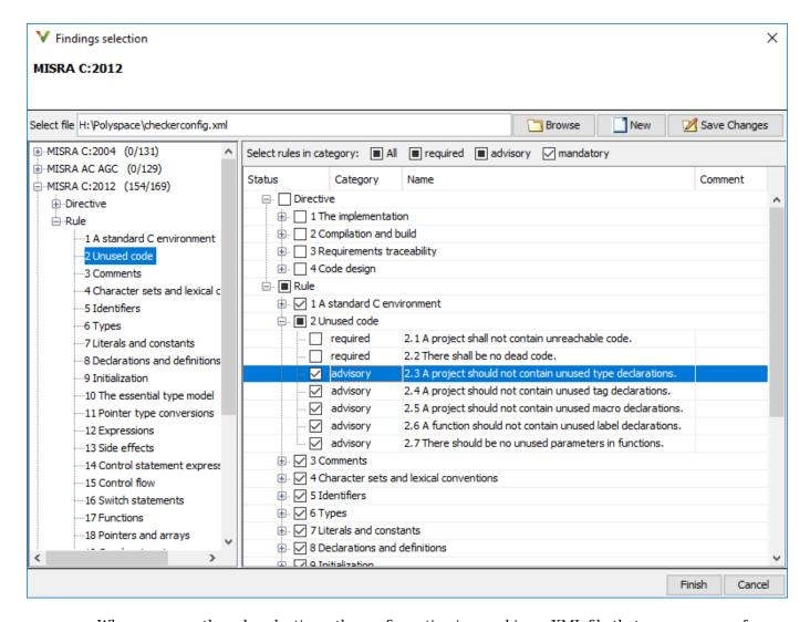
When you save the rule selections, the configuration is saved in an XML file that you can reuse for multiple analyses. The same file contains rules selected for all coding standards. You can reuse this file across multiple projects to enforce common coding standards in a team or organization. To reuse this file in another project in the Polyspace user interface:
