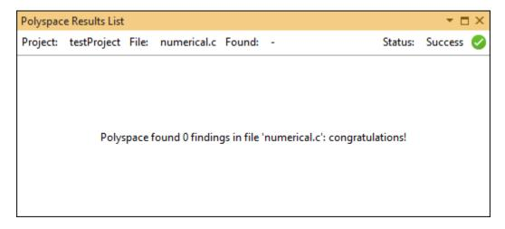
If the analysis failed to complete, you also see a status message indicating failure. For further diagnosis, check the analysis log within the IDE. For instance, in Visual Studio, open the Output pane, select **Polyspace** from the **Show output from** drop-down list, and check the messages. You might have to scroll up a bit to see the root cause of the failure.
