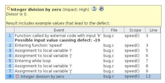
The tooltips on the defect show how the input value propagates through the code to eventually lead to one set of values that cause the defect.
