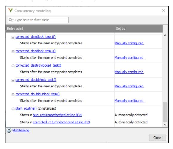
in the table, the functions are listed in the first column by order of decreasing priority. The second column shows how Polyspace detects each task or interrupt: automatically, manually from the Polyspace configuration, or from an external file.
