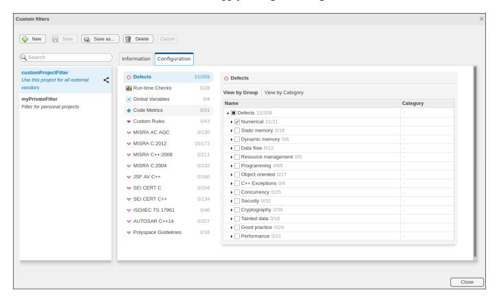
To create a new filter, in the **Custom filters** window, click **New** and then enter the filter name in the **New Custom Filter** pop-up window. You can optionally provide a description and enable the **Shared filter** checkbox to share the filter with other Polyspace Access users.
