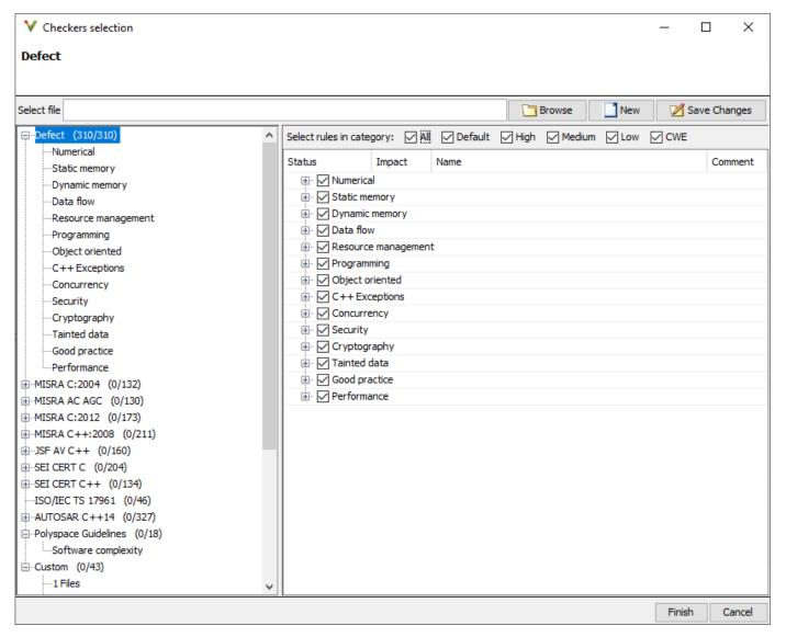
2 To create a new selection, in the Checkers Selection window, select the defect and the coding rule checkers that you want to activate. To modify an existing selection, click Browse, navigate to the existing checkers file and then modify the checkers selection.
